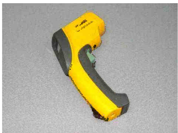
Photo 11 pyrometer to measure heat shrinkable sleeve external temperature - recommended
