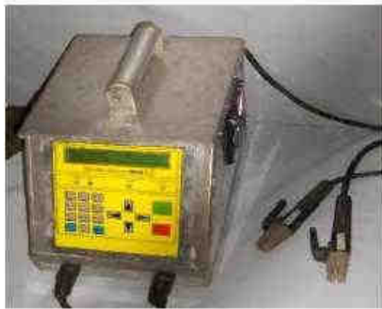
Photo 1 HG-2 Computer controlled welding machine to weld heat shrinkable joints
