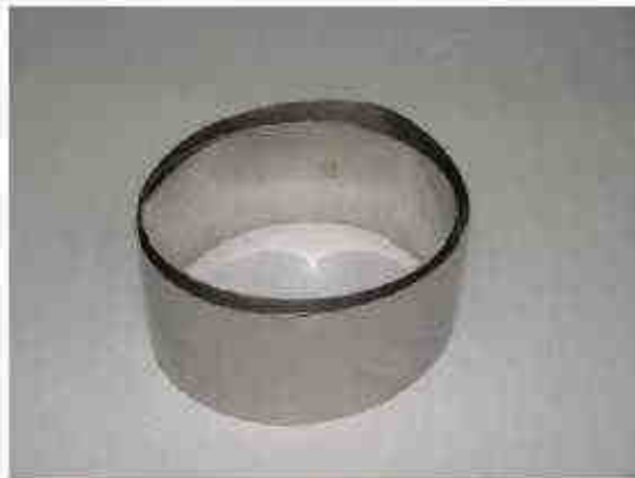
Photo 3 steel tightening separators
